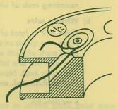
wire runs freely within spool flanges and slot of recording head, and that leader-thread is of sufficient length (at least 2 feet). Use special - minifon - leader-thread only.
