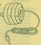
between wall socket and telephone plug. Insert plug of telephone transformer into socket (13) of - minifon P 55 -. Press Record key. Your two-way telephone conversation will now be recorded without interference.
