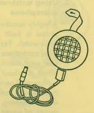
The volume control setting is dot to dash (• =) as long as the source of sound is not more than 3 feet from the microphone; during conferences at a distance up to 9 feet one notch lower (• =). For recordings at greater distances the volume control should be opened fully. At a distance of less than 2 feet do not speak directly into the microphone but always at an angle to or across the face of the microphone.
