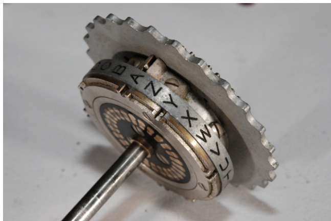
The left side of a wheel and the Ringstellung
