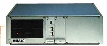
In this installation a telex terminal is connected to the central cipher computer. Since any standard telex can be used, this installation offers an economic solution for high quality autonomous cipher system. The comfort of the installation depends on the model of telex machine used.
