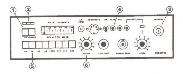
Operation is started by first setting all controls to 0 (zero) and putting all push button switches up.
