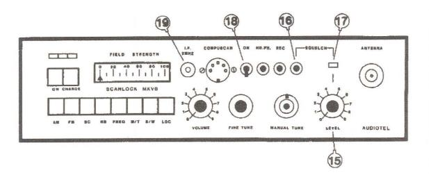
The SQUELCH circuit disables the audio output until the level of the signal acquired exceeds a certain level established by the setting of the LEVEL (15) control.
