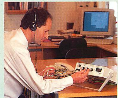
Checking for devices on a telephone line using TCM-03
