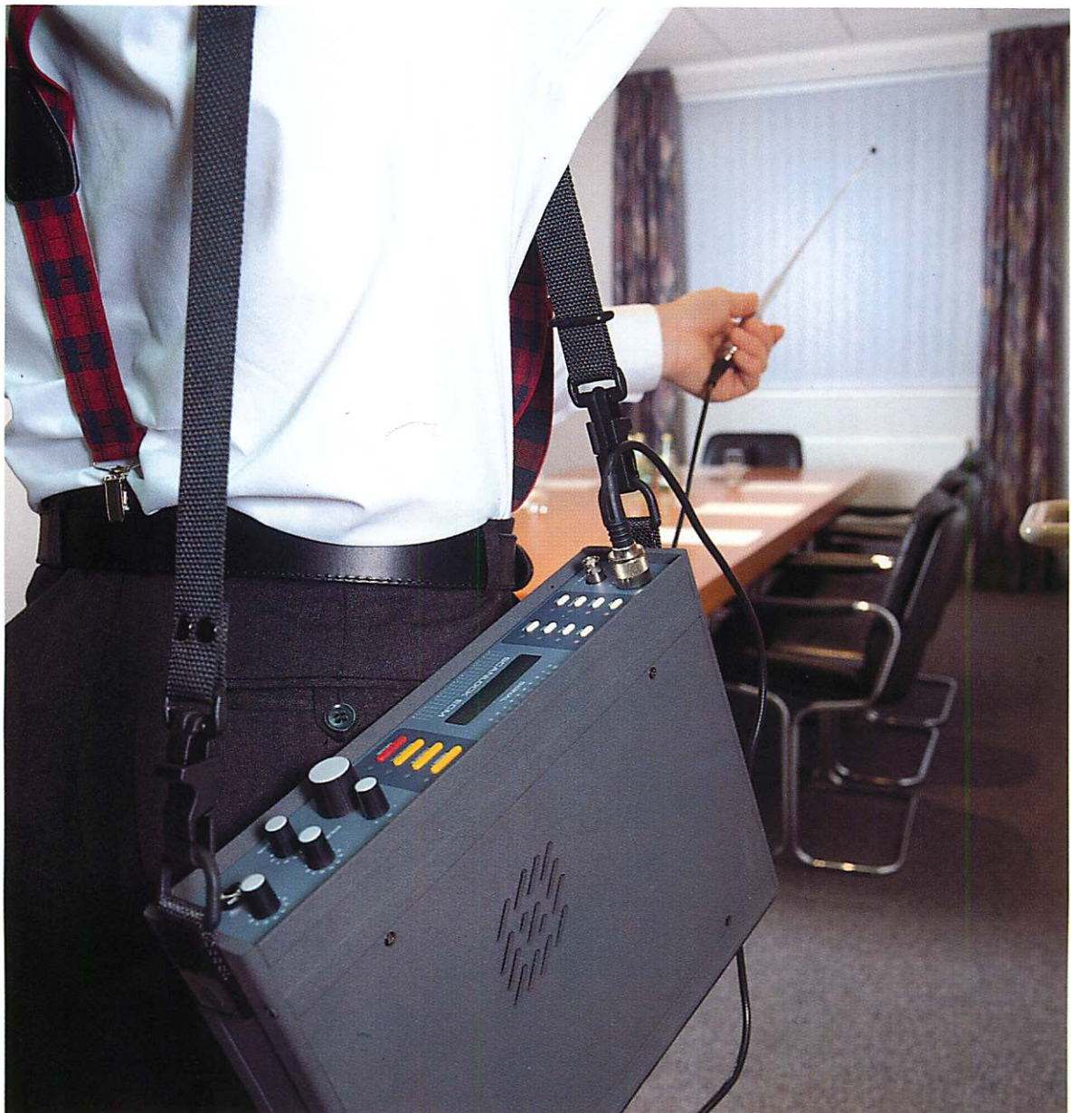
One of our team members starting a RF search using Scanlock ECM Plus
