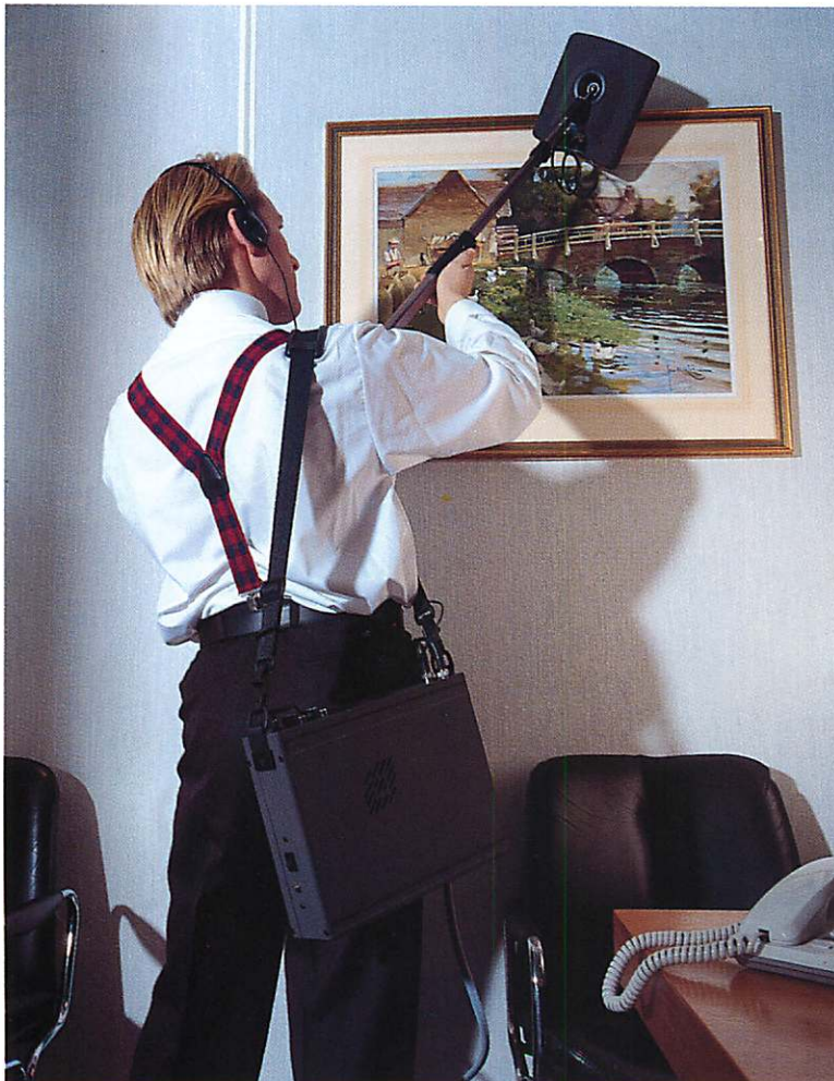
A sweep operator looking for suspect electronic devices using the Broom ECM non linear junction detector
