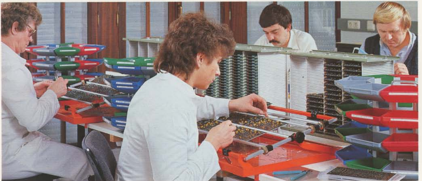
Prefabricated circuit boards are fitted with high-quality electronic components
